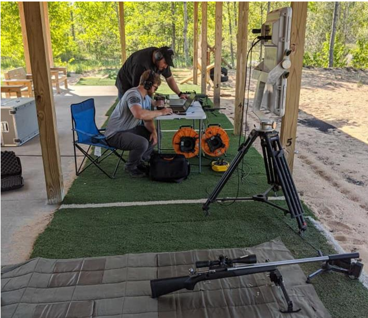
Figure 3. Applied Ballistics crew operating the doppler radar to measure MV and BC.
