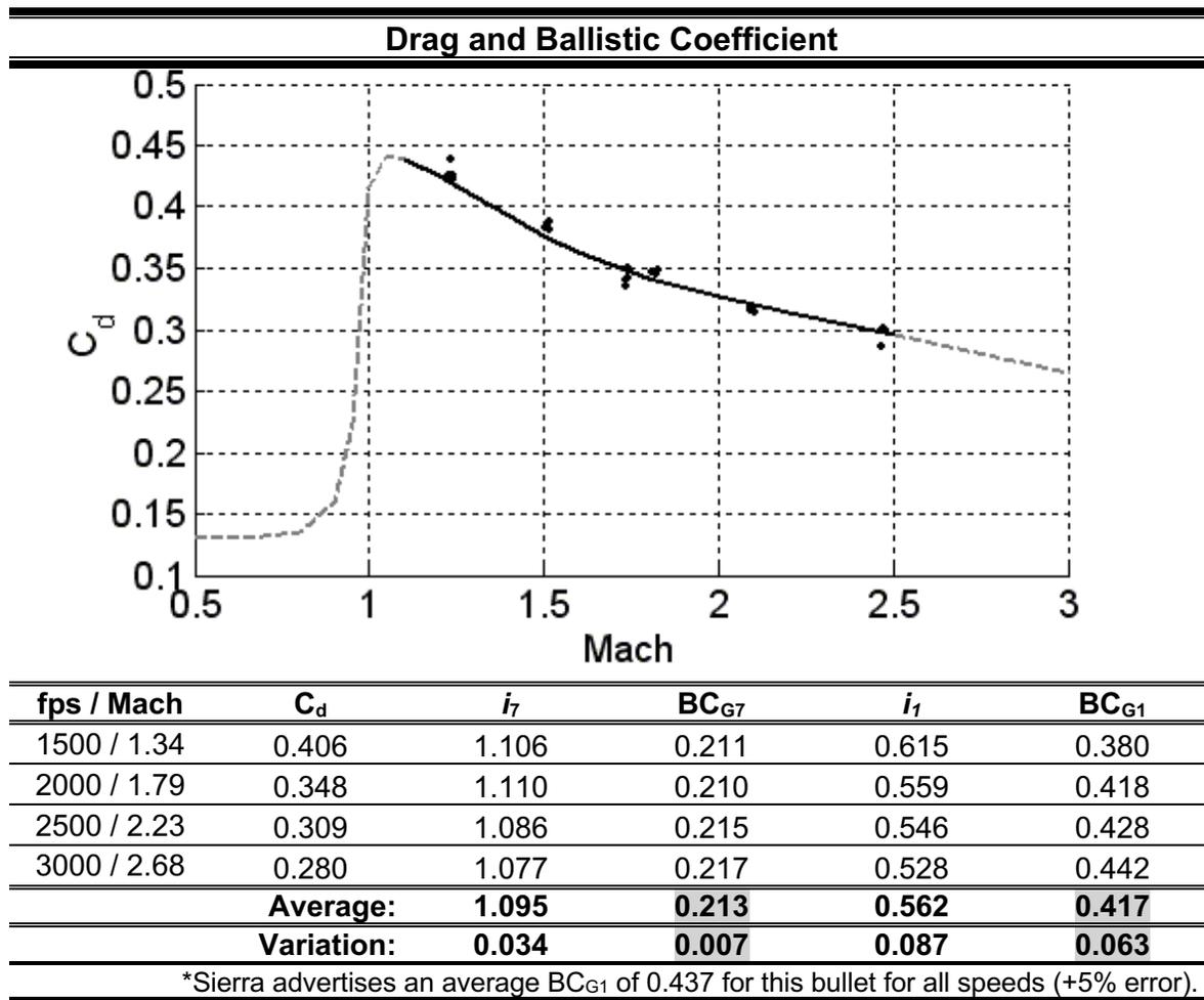
**Figure 2. Bullet drag coefficient and ballistic coefficient**
