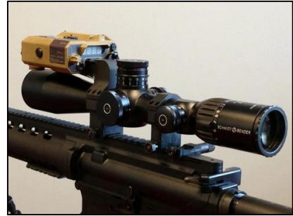
Figure 1. Example of a weapon-mounted LRF (Wilcox Industries RAPTAR). To
