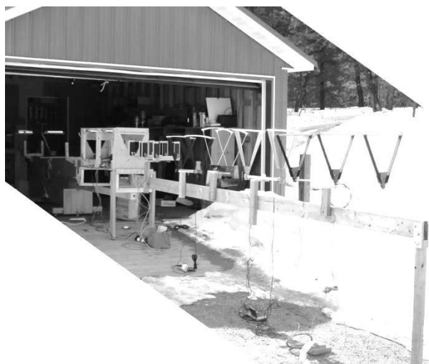
Figure 15.11. The array of chronographs as tested. In order from left to right: MagnetoSpeed (not visible), indoor Oehler on 12 foot rail, 4 foot Oehler built into light box, two PVM-21's, Pact,
