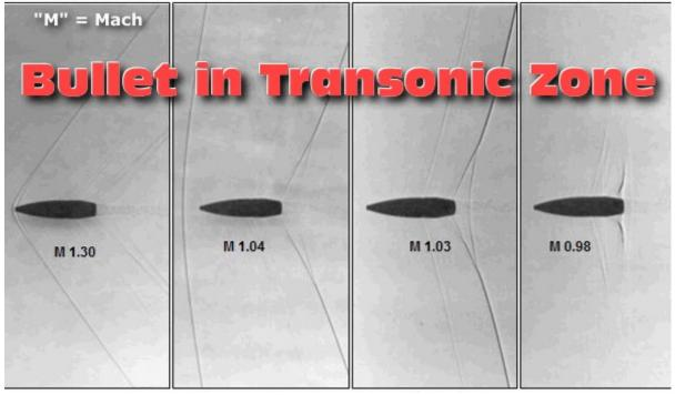
These four photos show the substantial changes in the shock wave and turbulence patterns for the same 7.5mm bullet at different velocities. The "M" stands for Mach and the numerical value represents the velocity of the bullet relative to the speed of sound at the time of the shot. Photos by Beat Kneubuehl.
