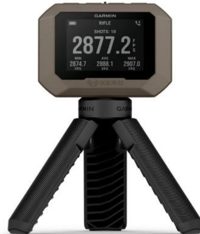
Figure 1. Garmin Xero radar chronograph and others like it have changed the uncertainty landscape in ballistics and with it, options for ballistic calibration are evolving.
